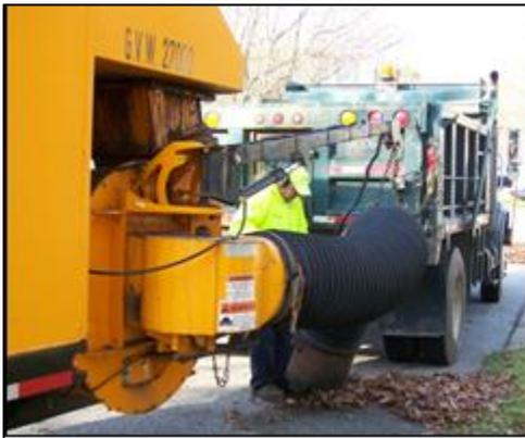
Visibility of the workers on foot is a critical component for a safe operation. In the picture on the left, the worker is between the leaf vacuum and the truck and out of the driver's sight.
