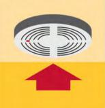
Put the alarm back on the ceiling or wall if it is less than 10 years old.
