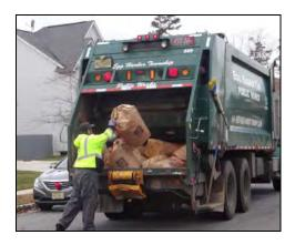
Leaf collection is a Mobile Work Zone. Establish traffic control according to the MUTCD. At a minimum, high intensity amber warning lights must be visible to motorists approaching from either direction.
